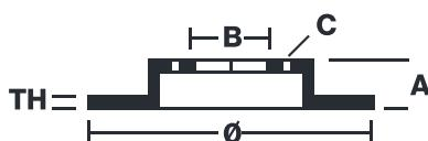
Diameter **302 mm** Thickness (TH) **12 mm** Height (A) **43 mm**
