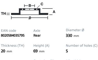
Brake disc type Ventilated Centering (B) Min. thickness 75 mm 18,4 mm
