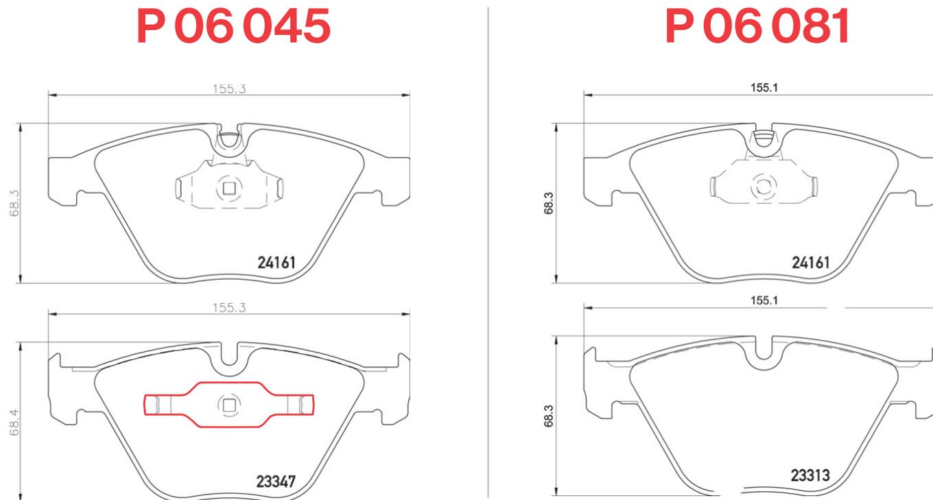
The difference is the lack of the piston clip on the pad with WVA 23313 vs 23347
