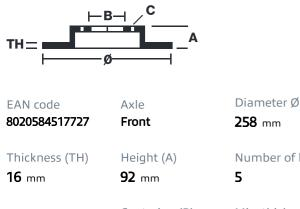
Centering (B) Brake disc type Solid **45** mm
