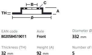
Brake disc type Centering (B) Ventilated 82 mm
