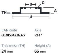
Brake disc type Centering (B) Ventilated 75 mm
