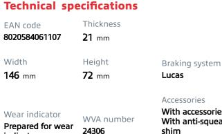
Accessories With accessories With anti-squeal shim With brake caliper bolts
