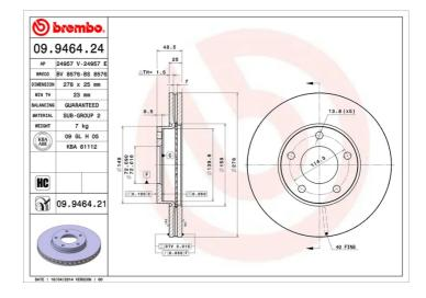
Tightening torque **103** Nm
