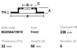
Brake disc type Centering (B) Ventilated 108 mm
