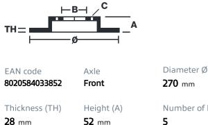
Centering (B) Brake disc type Ventilated **69** mm
