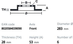
Brake disc type Centering (B) Ventilated 68 mm
