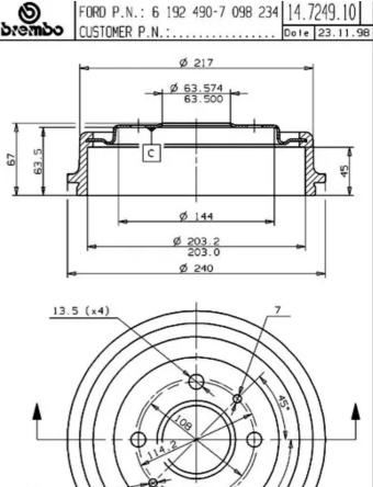
7.5 C MOUNTING FACE Max.DIA. 204 mm Weight 3.6 Kg
