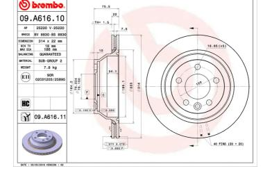
Tightening torque **170** Nm
