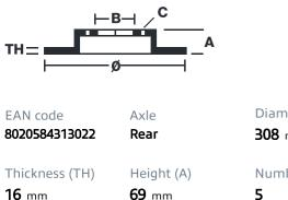
Centering (B) Brake disc type 96 mm
