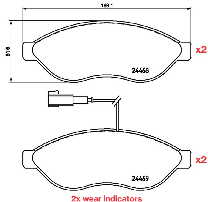
Existing stock of P 61 092 can be sold out. Please used only on vehicles equipped with one wear indicator.
