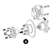
Fit the disc first, then the caliper.
