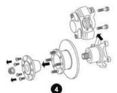
Remove the caliper first, then the disc.
