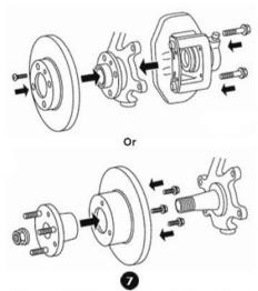
Fit the disc on the wheel hub, then the caliper.
