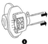
Disconnect the wear sensor if necessary. Remove the 2 pad pins.
