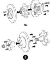
Remove the caliper first, then the disc
