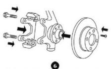
Fit the disc first, then the caliper holder.
