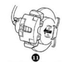
Reassemble the spring (retainer).
