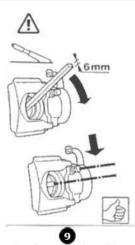
On models with a handbrake, push the pistons back, turning them and bringing the groove on the piston to the bleed screw axis.
