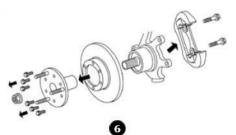
Remove the caliper holder first, then the disc.
