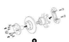
Fit the disc first, then the caliper holder.
