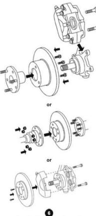
Fit the disc first, then the caliper.
