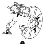
Dry clean the caliper and the wheel hub.
