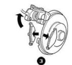
Turn the caliper and remove the pads.
