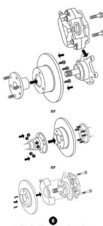
Fit the disc first, then the caliper.
