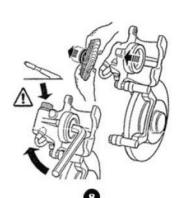
Push the piston back. On models with a handbrake, tighten the piston.
