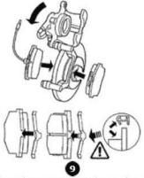
Introduce the new pads and turn the caliper.
