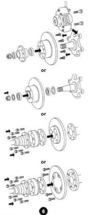
Fit the disc first, then the caliper.
