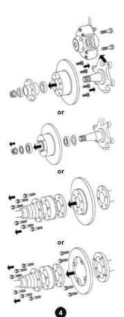
Remove the caliper first, then the disc.
