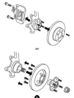
Remove the caliper first, then the disc.
