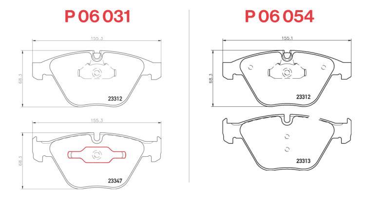
P 06 054 is applicable retroactively for all vehicles. The only difference between both parts is the finger side clips, which are removed now with P 06 054 for all vehicles.
